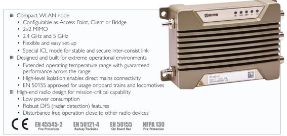
The Westermo RT-220-HV is a Wireless LAN Node for on-board and stationary applications. It ensures reliable connection for applications such as video transmission and TCMS, especially useful for transparent inter-consist links (ICL) with automatic reconfiguration.
